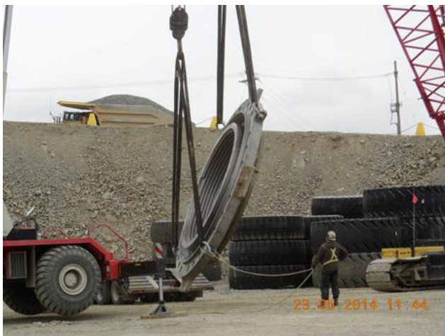
Adjustment ring being rotated for installation
